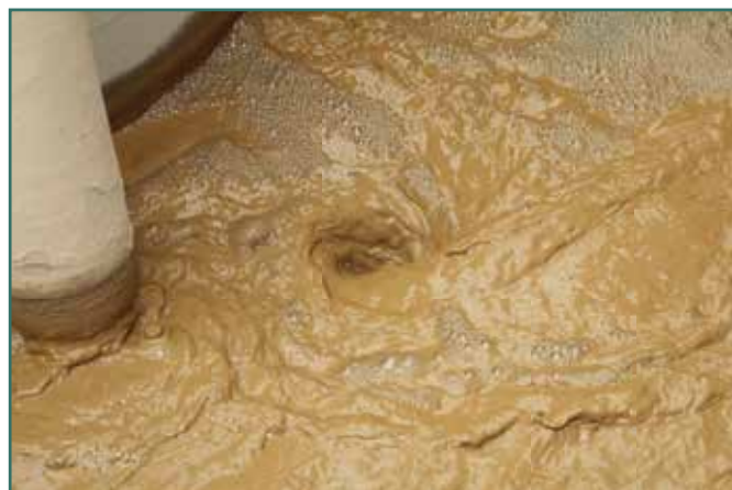
Suction vortex created by Varkie S55 in process plant sump while running
